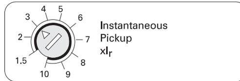
An instantaneous override function is provided on all trip units. It is nominally set at the short-time rating of the respective breaker frame size. This allows the breaker to ride through high fault currents up to its short-time capability, however, it is self-protecting above these values.
